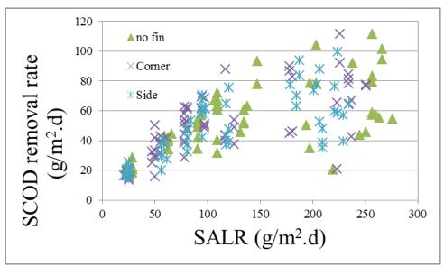
Figure 2: SCOD removal rates versus surface area organic loading rates
