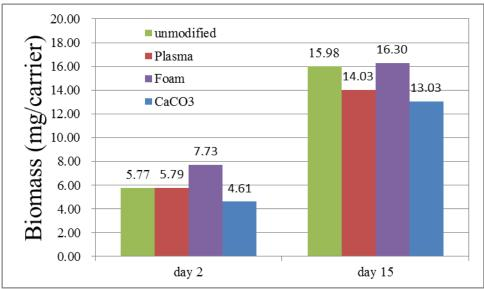
Figure 9: Biofilm growth during the initial biofilm build-up period
