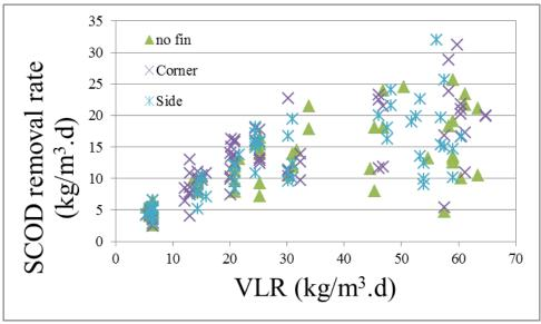
Figure 3: SCOD removal rates versus volumetric loading rates
