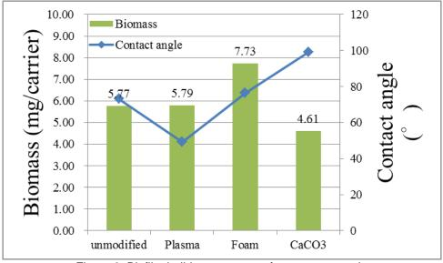
Figure 8: Biofilm build-up versus surface contact angle
