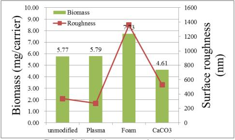
Figure 7: Biofilm build-up versus surface roughness
