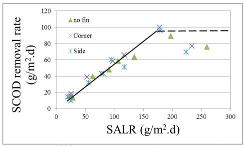
Figure 4: Averaged SCOD removal rates versus surface area organic loading rates
