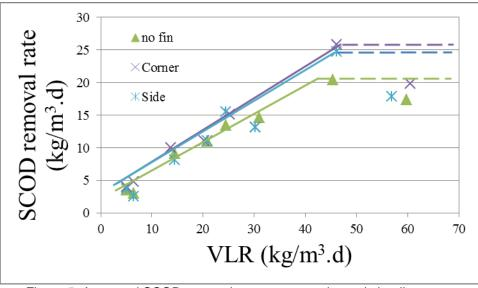
Figure 5: Averaged SCOD removal rates versus volumetric loading rates
