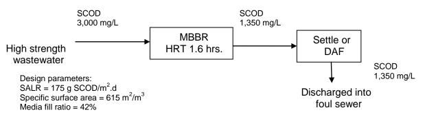
Figure 10: Treatment process using the new MBBR carrier
